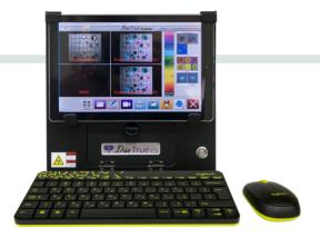
DIATRUE CS is a desktop diamond verification instrument for loose and mounted diamonds.
