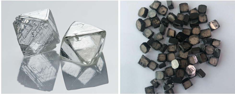
From left to right: Natural rough diamonds (photo by Leo Bieber), Unpolished CVD (Carbon Vapor Deposition) laboratory-grown diamonds
