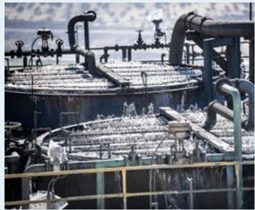
The coarse particle flotation process is already being used at Las Tórtolas, part of the Los Bronces copper mine, in Chile.
