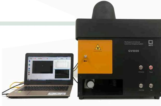
GV5000 is a desktop diamond verification instrument for loose and mounted stones designed to separate diamonds, synthetic diamonds and diamond simulants. GV5000 is manually operated and requires an operator to interpret the test results.
